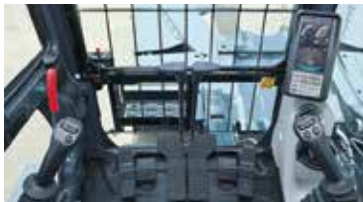
Suspension seat absorbs vibration Reclining seat has a wide recline angle
