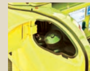
Removable fuel tank for easy washing
