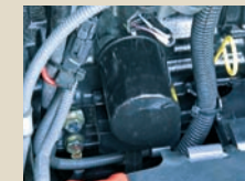
The engine oil filter has an oil catch pan, which prevents the engine oil from spilling when removing or installing the filter.
