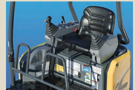
Three-pillar canopy compliant with ROPS and FOPS level 2
