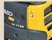
All steel guard for durability on the jobsite
