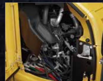
Control valve Cleanly mounted with easy access to test ports.
