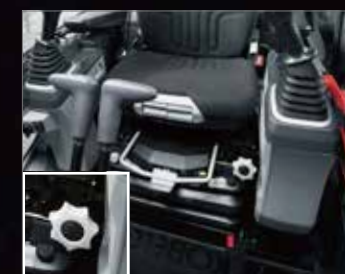
Adjustable Height Joystick Consoles The operator can adjust height of attachment control levers.
