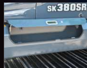
Ground level storage compartment access
