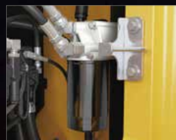
Fuel filters Main Filter / Pre-Filter with Integrated Water Separator.
