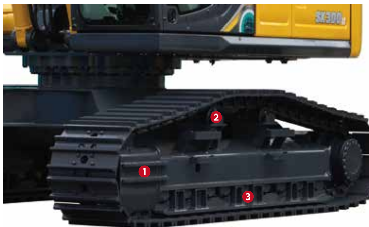
1 Reinforced guide frame * not applicable for SK500LC
