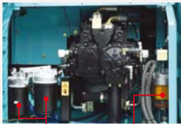
Engine oil filter Two large fuel filters (built-in water separator)
