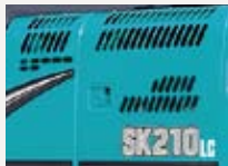
Ventilation Openings for tropical temperatures
