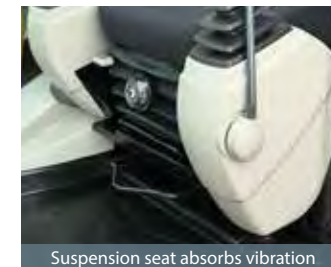
Suspension seat absorbs vibration
