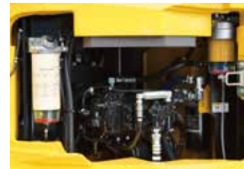
Fuel filter with built-in water-separator
