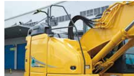
Handrail The handrail on the step side allows easy access to the maintenance port on the upper arm.
