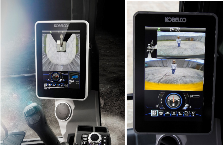
Photo Caption 2: The KOBELCO SK75SR-7 and SK85CS-7 feature a new 10-inch color monitor with a split-screen display function to customize operator viewing needs.
