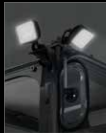
Forward and Left-Facing LED Light (Cab)
